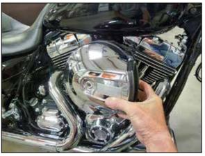
3. Remove air filter cover bolt and air filter cover as shown.
