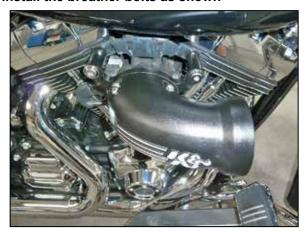
11. Install the K&N® intake tube with the gasket and provided hardware.
