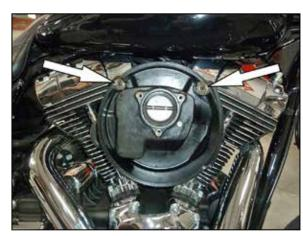
6. Remove the two breather/air filter base mounting bolts as shown.
