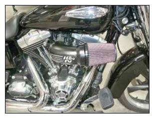
12. Install the K&N® air filter onto the intake tube and secure with the provided hose clamp.
